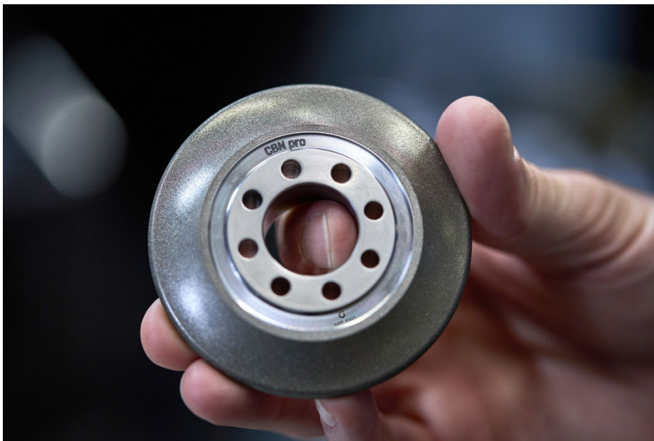
Picture 4: With CBN pro, the new tools from KAPP NILES, surface qualities of Ra < 0.2 \mu\text{m} can be achieved on the workpiece.
